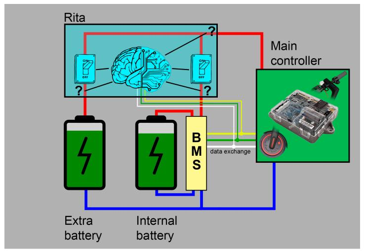
Rita analyzes voltages of the internal and external batteries, switching their positive power leads so that the charge does not flow from one battery to another, keeping the ability for the controller to consume current from both batteries and recover energy back when braking.
